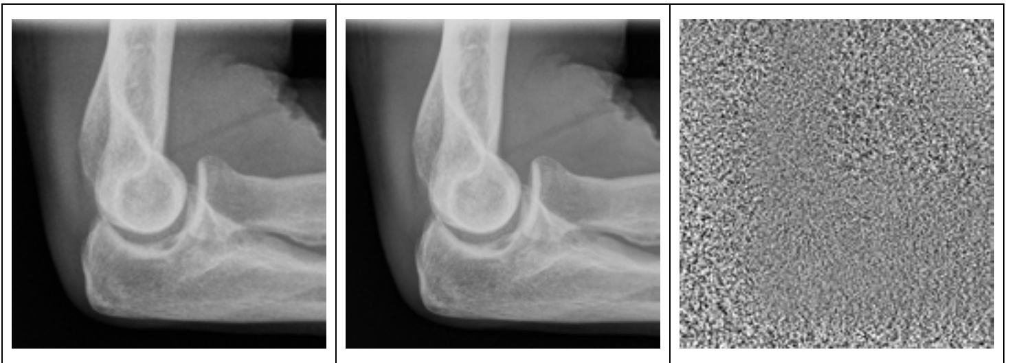
Figure 12. Adult elbow on DRX Plus 2530C: 55 kVp, 0.36 mAs, IEC EI 69. Left Image: EVP Plus default processing; Middle: EVP Plus with SNC; Right: Noise field.
